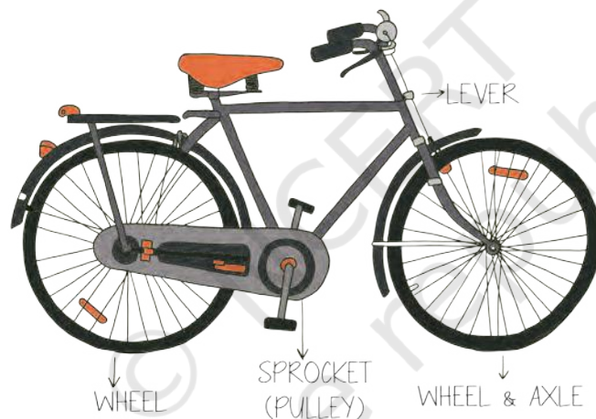
Figure 3.10: Parts of a bicycle
