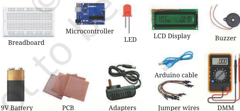
Figure 4.3: Electrical and electronic components
